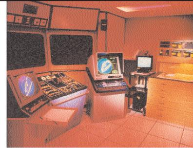
The Marine Institute's Navigation and Blind Pilotage Simulator trains mariners to navigate a vessel safely in restricted visibility with the use of instruments only.
