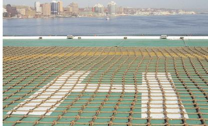
Heliport pad with scramble net aboard the Rowan Gorilla V offshore Halifax, Nova Scotia.
