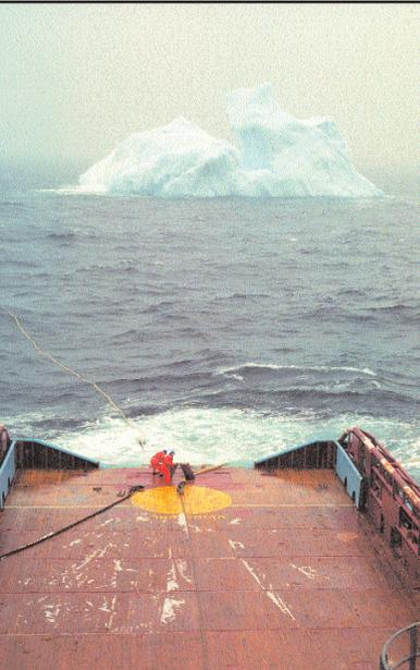
As part of Hibernia's ice management strategy, encroaching icebergs are "lassoed" with a heavy cable and towed by a support vessel into a different trajectory.
