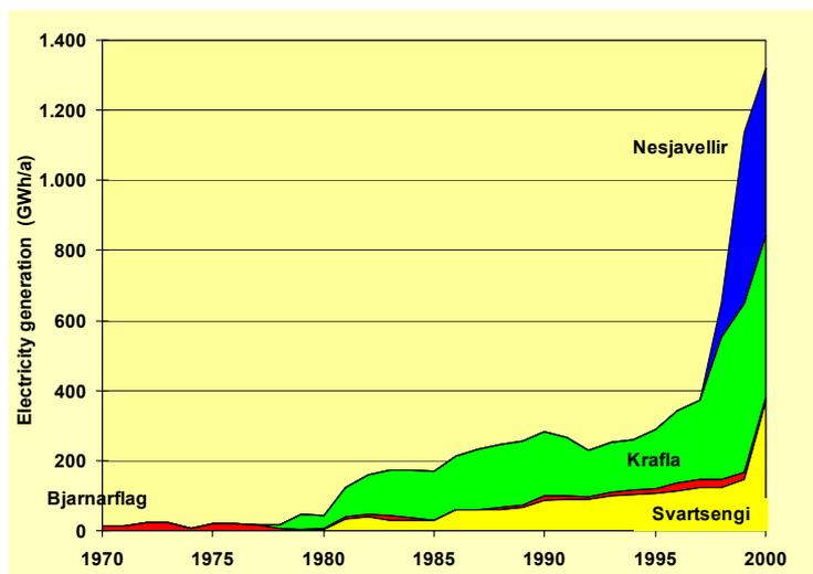
**Figure 4.** Development of electrical production from geothermal 1970 – 2000
